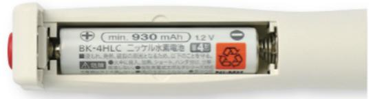
Battery : A4 Nickel hydride battery
